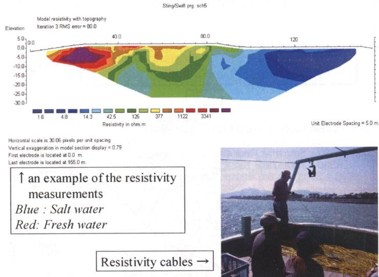
Fig.5 An example of the resistivity measurements
