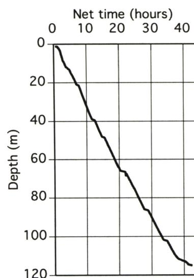
Fig.3 Cumulative drilling time (h) versus depth (m)
