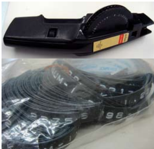
Tapewriter (DM1585-B, Orient Enterprise Co. Ltd.) and number-tag tape (9 mm width).
