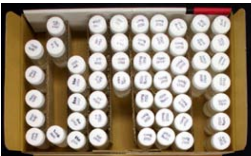
Tissue samples in screw-cap sampling glass bottles in a box. The box is placed in deep freezer after closing the lid.
