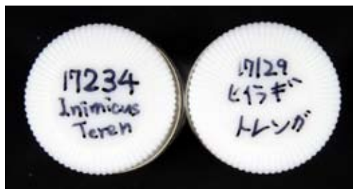
Data (specimen number, species name, and sampling site) written on a screw-cap.
