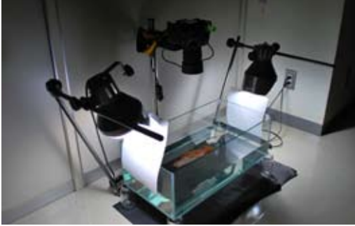
Figure 6. Photography technique for a specimen placed in water.
