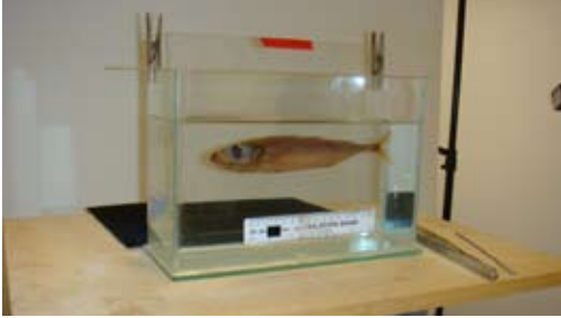
Glass aquarium seen from the front. The black board at the back of the aquarium is used for a photograph with black background.
