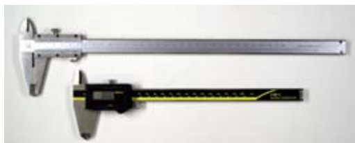
Caliper used in the Kagoshima University Museum. Above: VC-30, M-type standard caliper by Mitutoyo, Japan. Below: CD-SC, series 500 ABS digimatic solar caliper by Mitutoyo, Japan.
