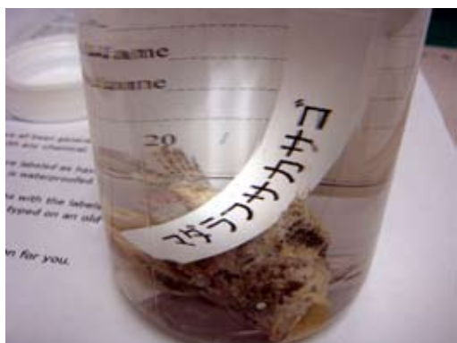
Specimen fixed in 99% ethanol (for DNA analysis). Label is printed using a thermoelectric printer, which prevents deterioration or loss of print.
