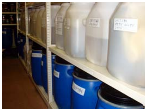
Storage containers for medium to large specimens. Upper row: 20-L wide-mouthed BB-type bottle without stopper cock. Lower row: 25-L plastic drum. Label the front side with white vinyl tape, and write the family number and species name with alcohol-resistant Sharpie Fine Point pen (sold in Europe and the United States).
