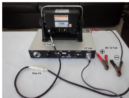
Figure 12. Power cable connection.
