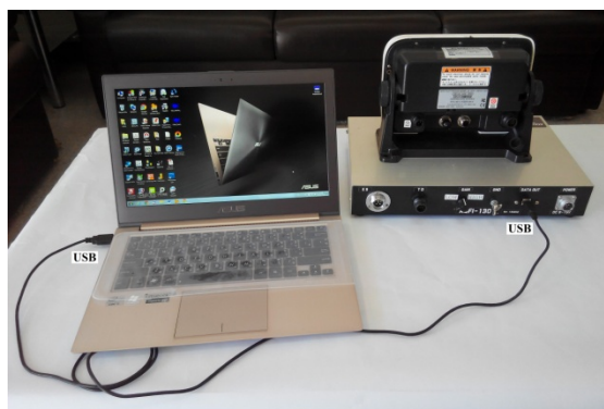
Figure 15. Data output connection.
