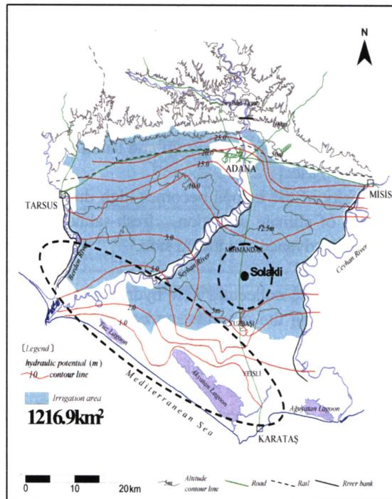
Fig.5 Irrigation areas and potentiometric contour map in September 1983.
