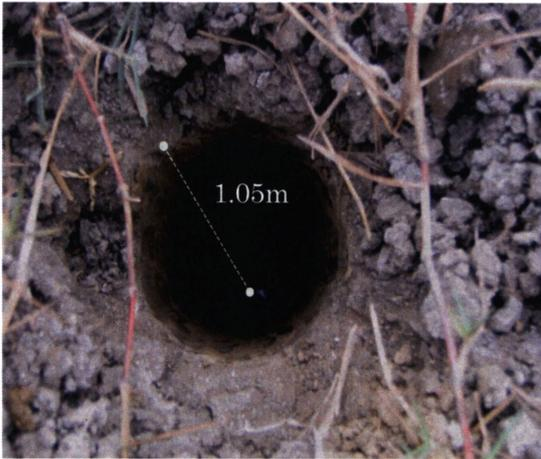
Photo.1 Shallow groundwater level in a bore hole on a salinity field
