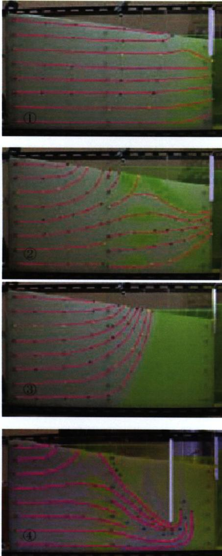
**Figure 3** Experimental results for: ①lowsea water level without drainage, ②highsea water level without drainage, ③highsea water level with drainage, ④high seawater level with drainage and a barrier
