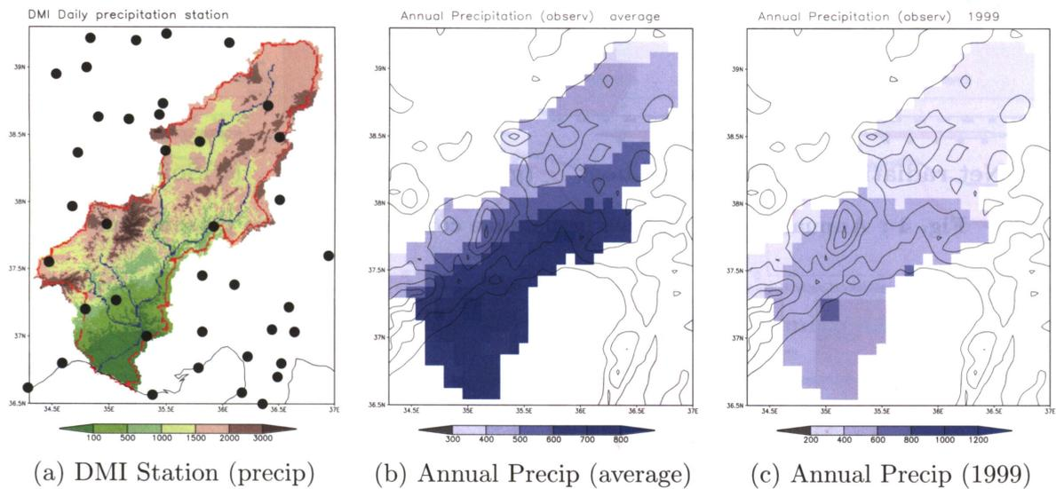
**Fig. 2 : Surface meteorological station and gridded precipitation data**
