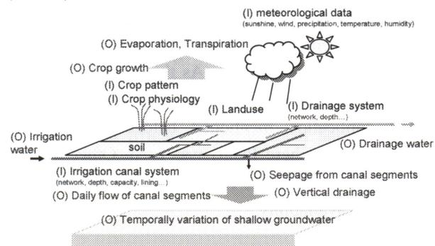
Figure 1: Input (I) and output (O) of IMPAM
