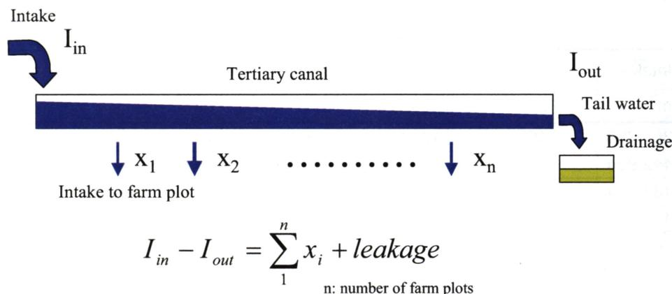
**Fig. 4 .** Water intake and tail water measurements
