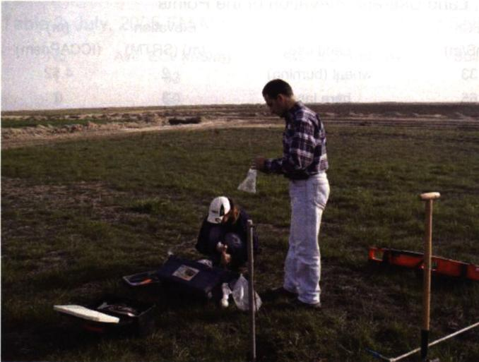
Figure 6. Soil sampling and EM measurements
