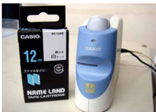
Thermoelectric printer (Name Land; CASIO) for printing labels for specimen bottles. We use black ink for normal specimens and red ink for type specimens. Further, we use 12-mm-wide tape for 0.5- to 3-L specimen bottles and 9-mm-wide tape for 0.25-L specimen bottles.
