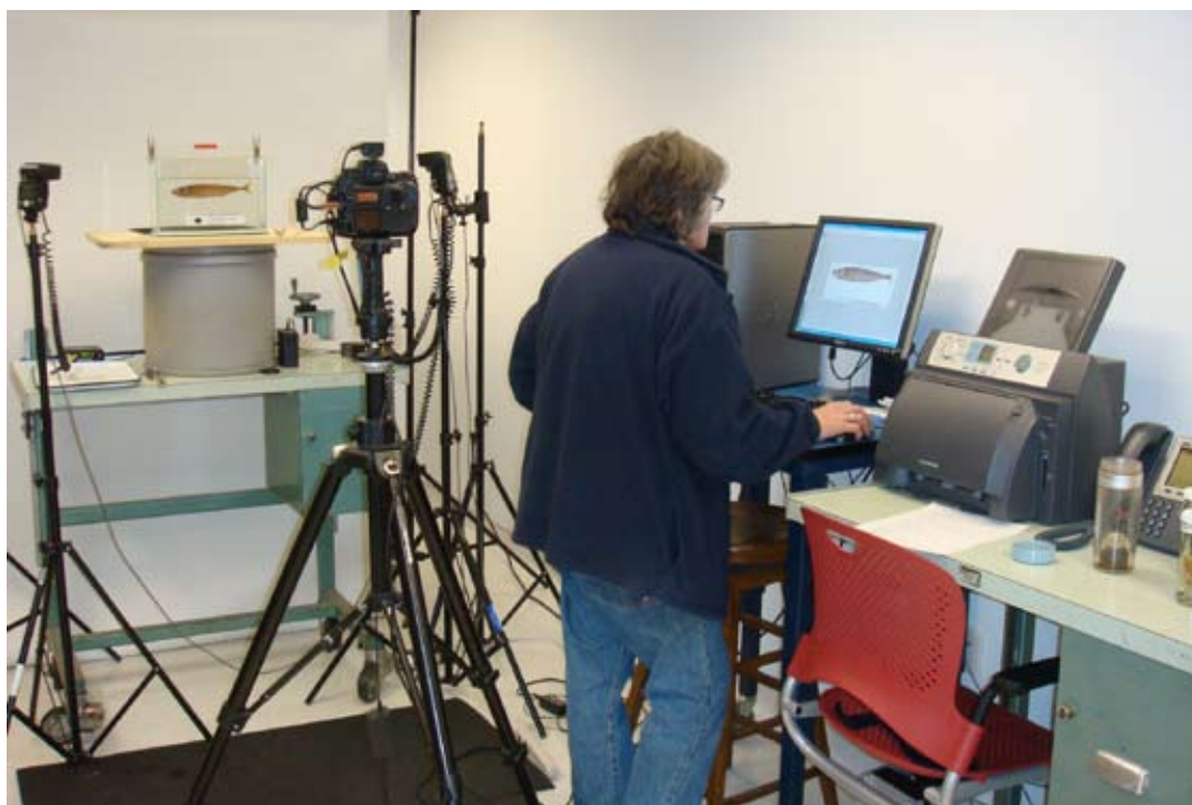
Specimen photography room at the Museum Support Center, Smithsonian Institution National Museum of Natural History. Side-view photography of the type specimen in progress. Camera is fixed on a tripod, and flash lamp is used for lighting. The photographed image is scanned directly into the computer.
