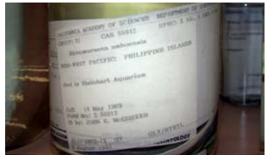
Specimen label printed with dot impact printer and alcohol-resistant ink. The print is too light and hard to read (photo by D. Catania).
