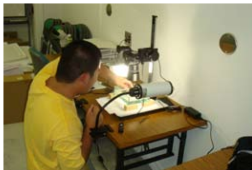
Close-up copy stand, light, and glass aquarium for small specimens.
