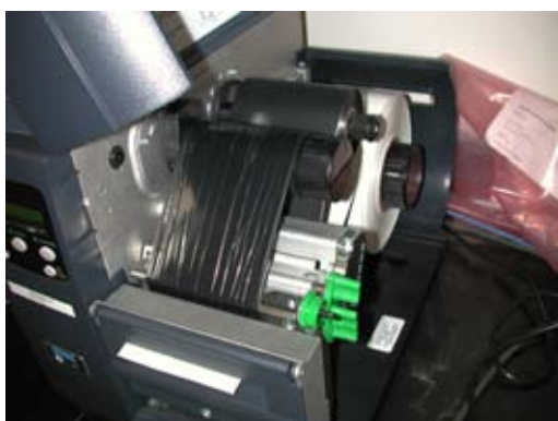
Datamax I Class Thermal Printer. In the photo, the black roll is the ink ribbon and the white roll is acrylic-coated paper (Photo by D. Catania).
