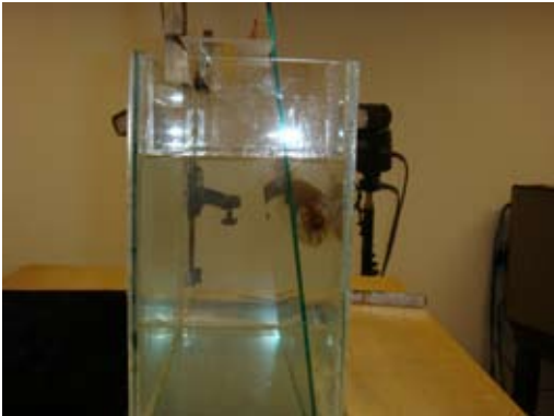
Glass aquarium seen from the side. Fish is stabilized by placing between a glass board and front side of the aquarium.
