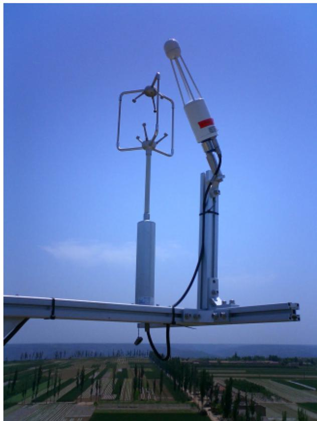
Fig. 2 A set of ultra-sonic anemometer-thermometer and infrared H<sub>2</sub>O/CO<sub>2</sub> gas analyzer installed on the tower.
