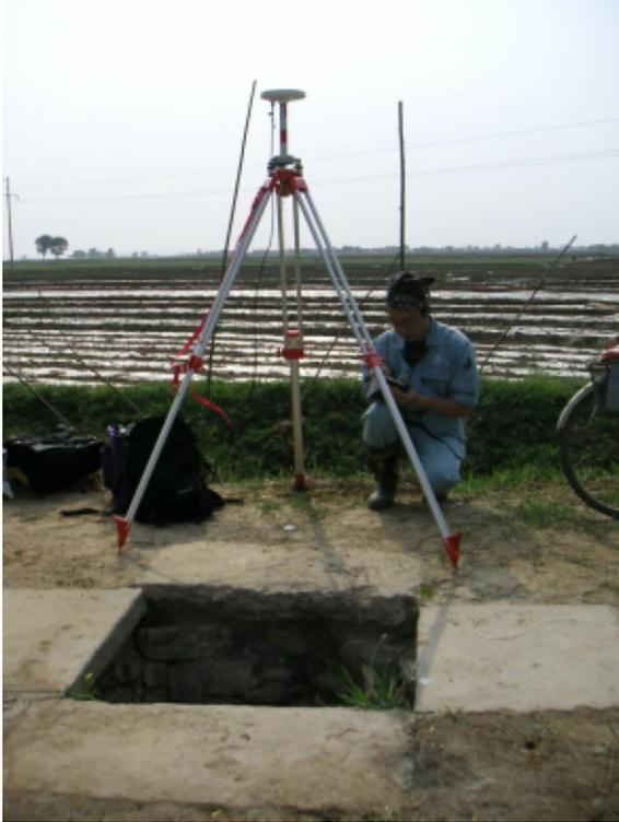
**Fig. 2** Static GPS survey.
