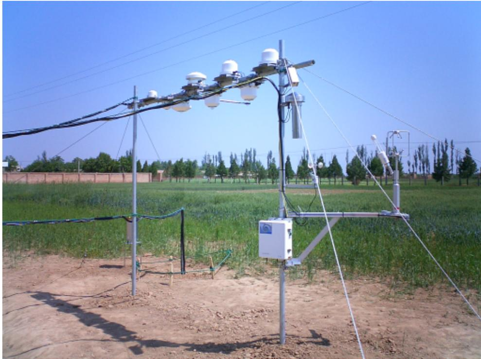
Fig. 3 The radiation measurement system installed on the ground surface. A set of ultra-sonic anemometer-thermometer and infrared H<sub>2</sub>O/CO<sub>2</sub> gas analyzer are also shown.
