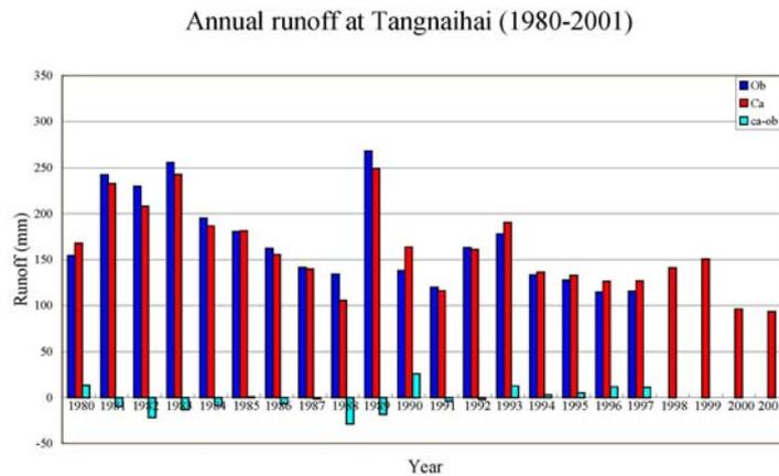
**Figure 4 Annual runoff and its error between simulation and observation at Tangnaihai gauge from 1980 to 2001.**
