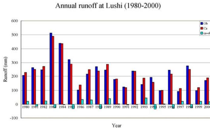
**Figure 6 Annual runoff and its error between simulation and observation at Lushi gauge from 1980 to 2000.**
