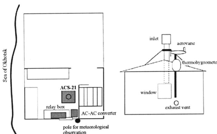
Fig 2. Schematic view of the aerosol sampler
