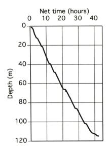
Fig.3 Cumulative drilling time (h) versus depth (m)
