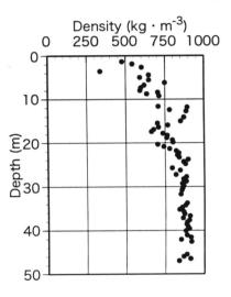
Fig.5 Bulk density profile of the ice core from the surface to 50 m depth
