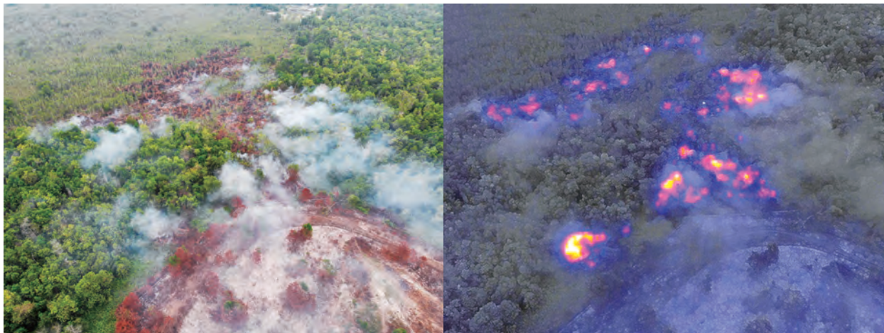
Figure 1. Regular image (left) and one overlaid with thermal data (right) taken by a Mavic 2 Enterprise Dual camera (November 2019 in Palangka Raya).
