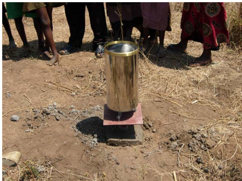
Fig. 2: Photograph of a rain gauge used in this study. The data logger is installed inside the gauge.
