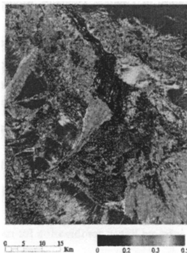
Figure 4. The image of albedo generated with the band integration method presented in the context (subset image of albedo with 2110*1794 pixels around Zhangye )
